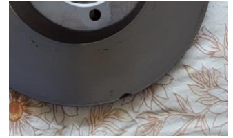
And here's the offending chip on the edge of the rotor, which appears on the reverse face as well.
