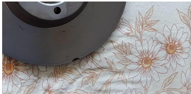
And here's the offending chip on the edge of the rotor, which appears on the reverse face as well.
