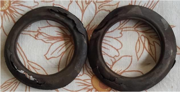
Yes, this is what the old calliper dustboots looked like, No wonder the pistons were u/s. I sourced a new genuine calliper kit from USA, through Ebay.
