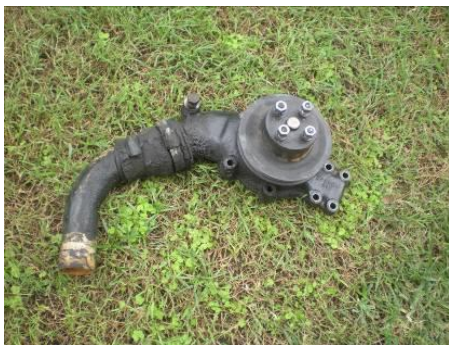
The hose between the water pump and the intermediate pipe was difficult to source.
