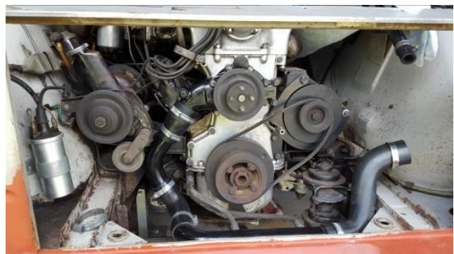
And here's the installed water pump, showing the bottom hose configuration.
