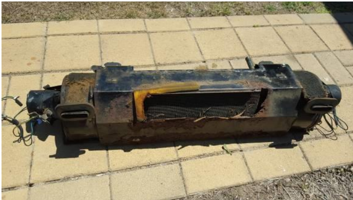
The rusted-out heater box.....
