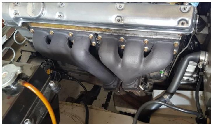
...and after welding, sandblasting and painting.
