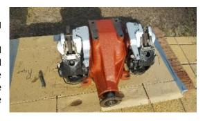
The diff was cleaned and painted. Calipers reconditioned and the rotors machined. The handbrake calipers (centre) were dismantled and cleaned, but were in surprisingly good condition. The diff pinion oil seal leaks, and needs changing, but for now I can't get the 1½" nut off, so I'm leaving the joy of that procedure for later.
