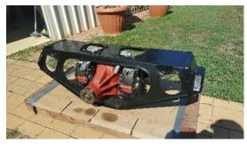
with the wheel bearings and fulcrum shafts. I read up about setting the bearing end-floats and fulcrum shaft pre-loads, and thought I had it sussed, but suffered a crisis of confidence. Luckily Alan Lincoln rode to the rescue on his trusty steed (XJ6 S3), not only walking me through the measuring and calculation process, but also machining the correct spacer for the wheel bearings.
