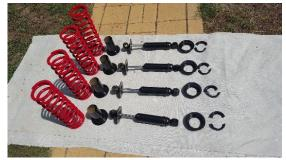
bench, they were cleaned and painted, the springs powder-coated fire-engine red to match the front springs.
